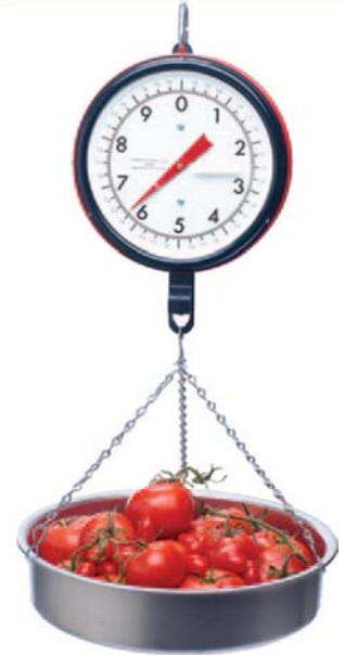
▲ You can use a spring scale to measure weight.
