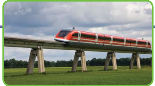
▲ Maglev trains use magnets to lift them above the tracks while moving.
